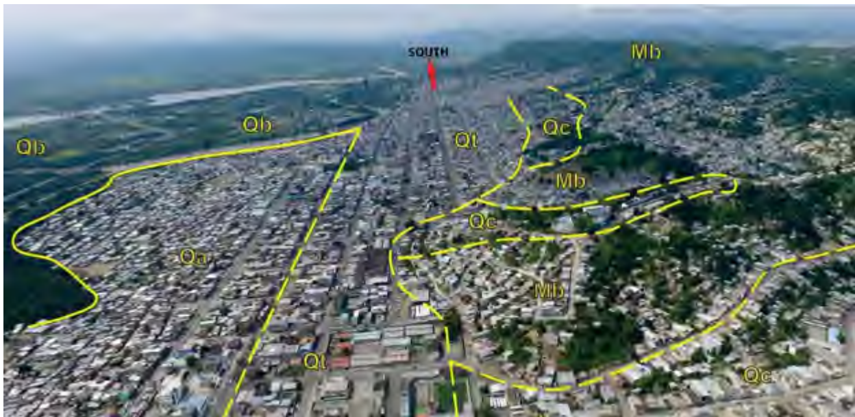
Figure 5. Spatial distribution of geomorphological features for the city of Esmeraldas, with the following abbreviations: Qa, floodplain alluvial plain; Qb: islet of flood barriers; Qt: alluvial terraces; Qc: quaternary colluvial soils; Mb: hills formed by lithologies of the Miocene and Pliocene formations Onzole and Bourbon. Photo City Courtesy: "photo & video drone Esmeraldas". Flood-prone geomorphological features may be considered to estimate the maximum run-up of tsunami waves.
