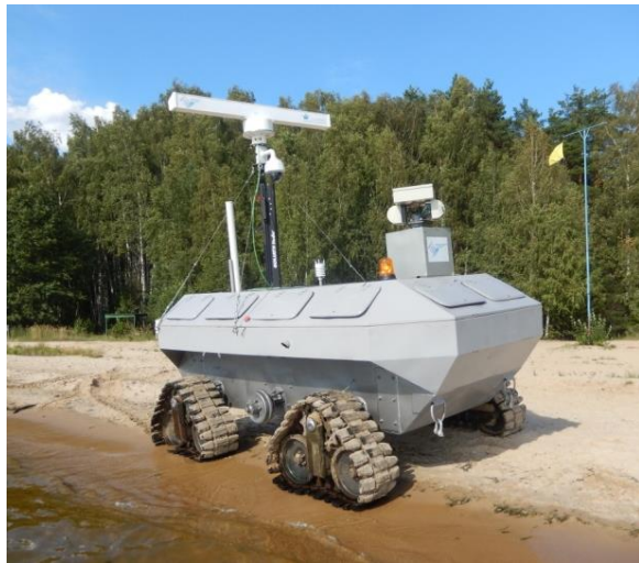
Fig. 1. Autonomous mobile robotic complex: 1 – LIDAR LMS511Pro; 2 – OS-103 positioning system antennas; 3 – Vaysala WX520 weather station; 4 – Rocket M2 omnidirectional Wi-Fi antenna; 5 – AXIS Q6045-E video camera; 6 – MRS-1000 circular view radar
