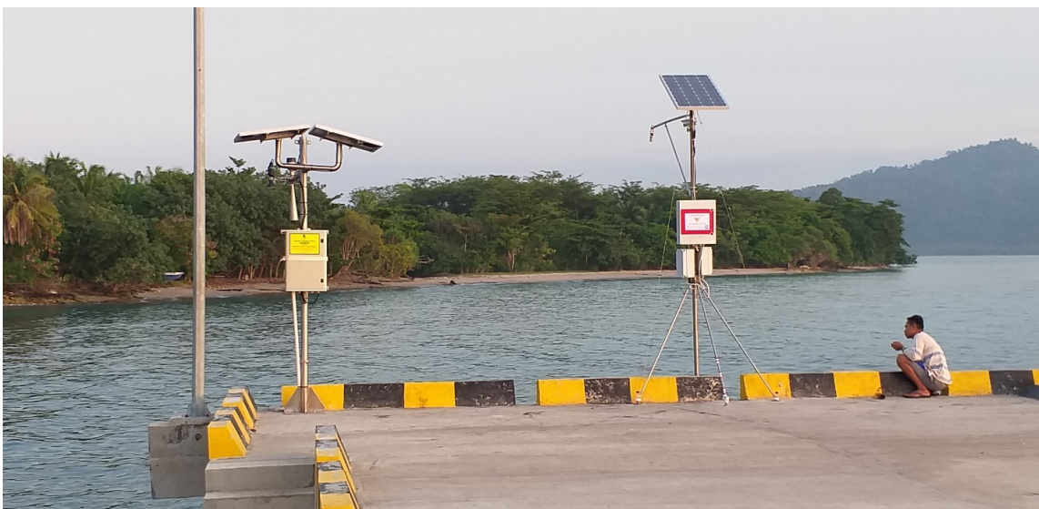
Figure 8 – On the left the BIG tide gauge installation and on the right the IDSL one, both on the Sebesi Port.
