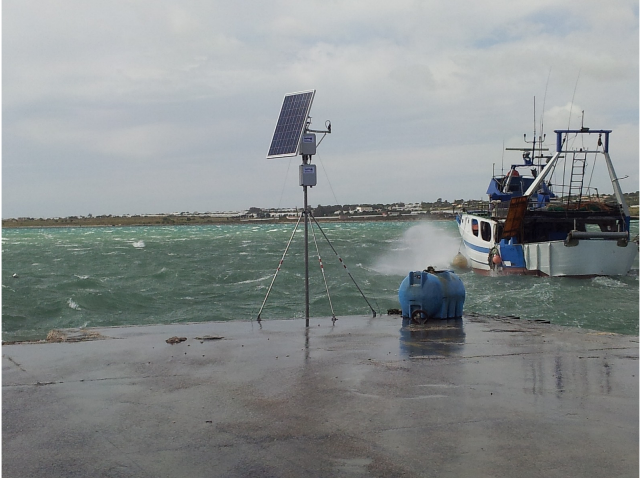
Figure A.1 - Typical installation of an IDSL device (Portopalo di Capo Passero, Italy)
