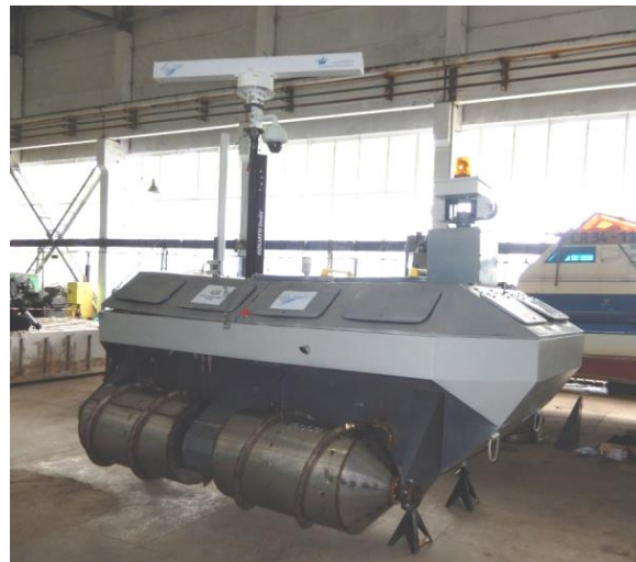
Fig. 1. Autonomous mobile robotic complex: 1 – LIDAR LMS511Pro; 2 – OS-103 positioning system antennas; 3 – Vaysala WX520 weather station; 4 – Rocket M2 omnidirectional Wi-Fi antenna; 5 – AXIS Q6045-E video camera; 6 – MRS-1000 circular view radar
