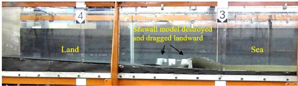
(b) The seawall was damaged by tsunami
