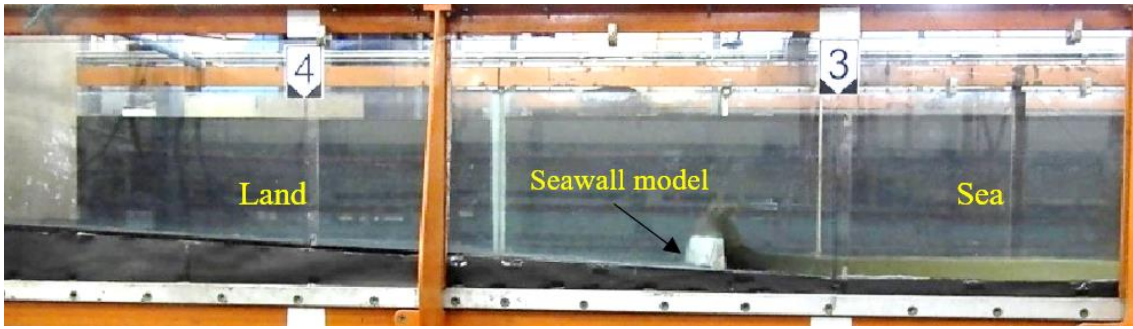
(a) The tsunami hit the seawall
