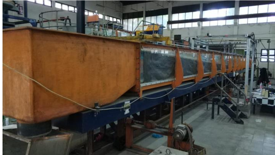
Figure 14. The flume equipped with dam break generation facility
